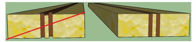
6. Use a stop block, when sawing your strips, to ensure all are of a consistent width.
