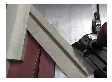
7. Use a gluing jig when assembling/gluing the zigzag. It needs a straight edge along the bottom where all the strip points can rest. One end of the jig needs to have a vertical member to ensure all strips are perpendicular. Glue up the whole zigzag at once. Make sure all points touch the strait edge along the bottom of the jig and make sure all strips lie flat against the face of the jig.
