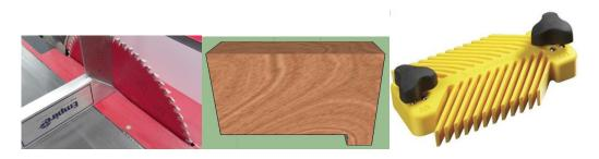
3. Make sure all your stock is straight, constant in thickness, and has sides that are cut at 90 degrees.
